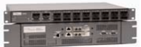
OptiView™ Link Analyzer and an 8 port in-line fiber tap.
