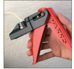
4. Ensure jack is completely and securely inserted in jack holder bed with IDC slots facing the blades.
