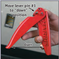
1. Make sure handle is in open position. Push handle and blade toward each other.
