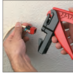
3. Insert jack in JackRapid front first with IDC slots facing blades of JackRapid.
