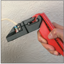
5. Pull trigger completely and remove excess wire prior to releasing trigger.
