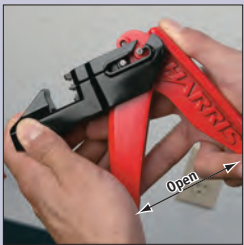
1. Open tool handle and move lever to pin #1 "down" position.
