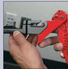
3. Make sure handle is open. Once pin #1 has been inserted, slide pin #2 into blade head.
