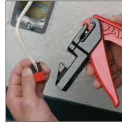
7. Release handle and remove jack from JackRapid tool. Visually verify proper termination.
