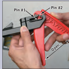
2. Angle handle so that pin # 2 will slide out first. Then slide out pin # 1.
